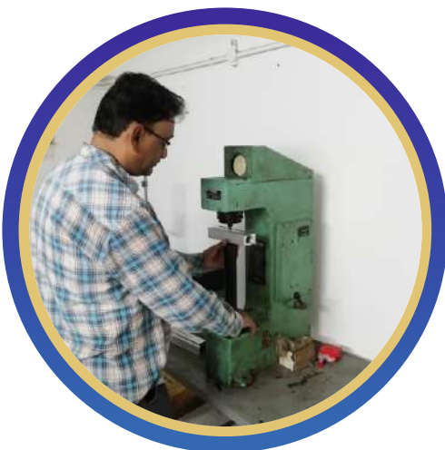
Hardness Testing of Aluminium Section
