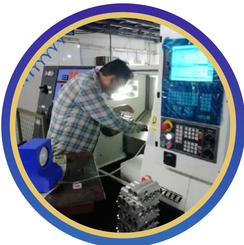
Online Bore Measurement With Air Gauge
